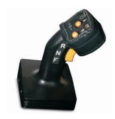
STIC™ Steering Control. STIC™ combines directional selection, gear selection and steering into a single lever for maximum responsiveness. Simple side-to-side motion turns machine right or left. Transmission shifting (forward/neutral/reverse) is controlled using a three position rocker switch. The thumb operated upshift and downshift button controls manual shifting.
