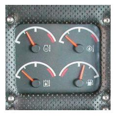
• **Gauge Cluster.** Maintains a constant display of vital machine functions, including: engine coolant temperature, brake oil temperature, air system pressure and fuel level.
