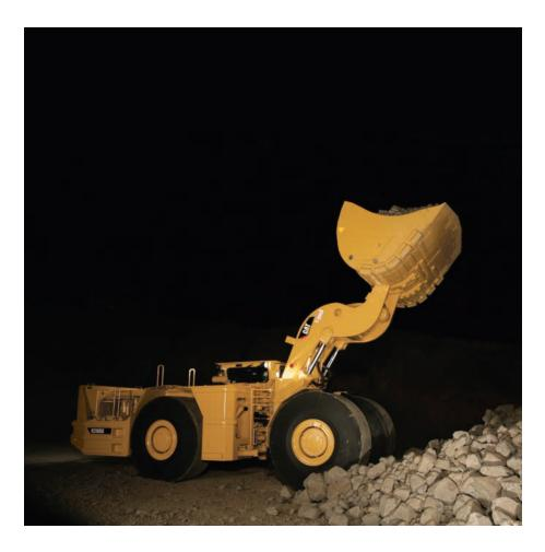
**Pilot Controls.** Low effort, pilot operated joystick implement control with simultaneous lift and tilt functions optimizes operating efficiency.
