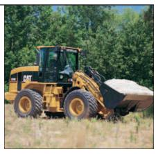
**Biodegradable Hydraulic Oil.**Caterpillar biodegradable hydraulic oil can be used in the 924G, providing an environmentally-sound alternative to mineral-based oils.
