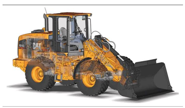
Caterpillar Engine. The six-cylinder, 3056E direct injection, turbocharged (DIT) engine with air-to-air after cooler (ATAAC) has a proven reputation for reliability, durability and performance. Fuel injection is electronically controlled for precise timing.
